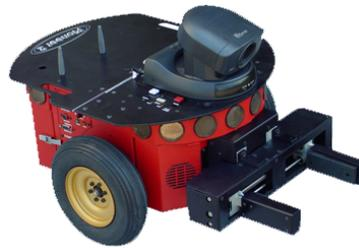
Fig. 5: A typical prototype of Pioneer 2-DX robot with gripper.
